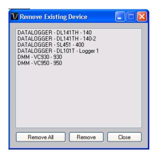
To remove a device, click the device in the list and click on the Remove button. Click the Remove All button to remove all devices at the same time.
