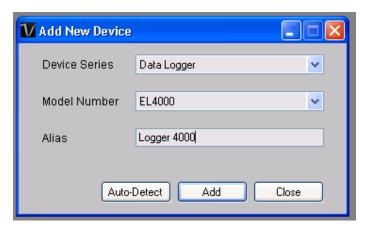
Select "Data Logger" in Device Series and "EL4000" in Model Number, input an alias and click "Add" to continue.
